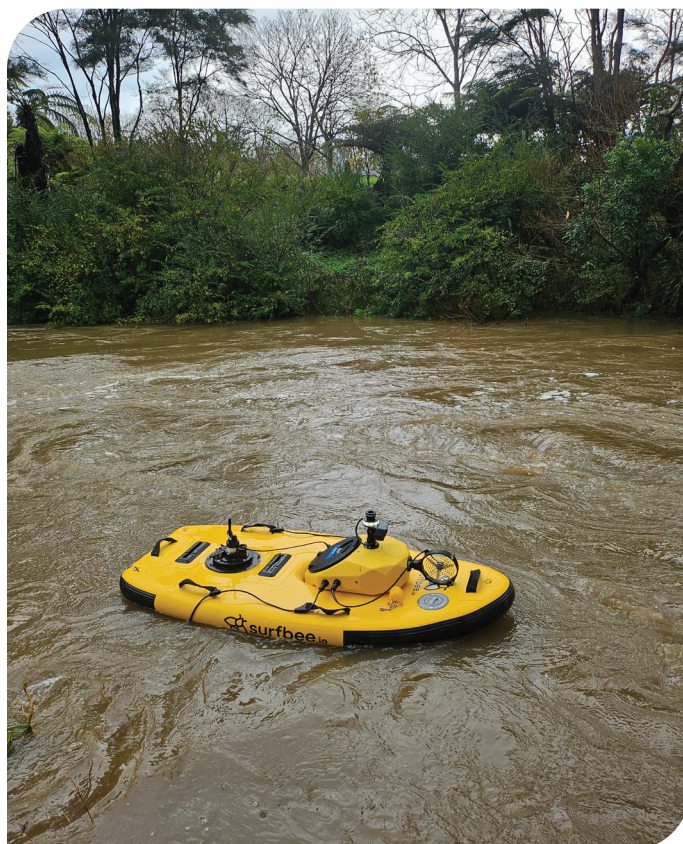
The SonTek-RS5 and Surfbee collect discharge data during a flood event in New Zealand. During El Niño, stronger westerly winds can bring wetter conditions to western regions while increasing hydrologic variability across the country—reinforcing the need for safe, adaptable flow-monitoring methods. Photo credit: Graham Andrew, ENVCO.
