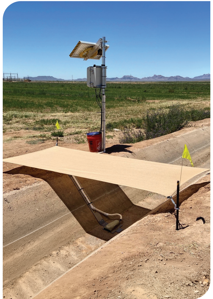
The SonTek-IQ supports continuous flow monitoring in an irrigation canal during dry conditions in Yuma, Arizona. Drought planning is not only about measuring less water—it is about maintaining reliable data as flows decline, operational demands shift, and every available supply becomes more important.
