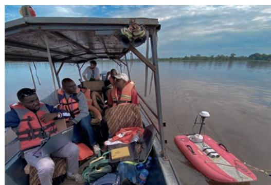
Technician Matti Barthel navigating through floating islands and traditional dugout canoes during discharge measurement of the Congo main stem. Photo: T. Drake
