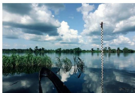
Ruki river gauge height after final installation. Together with the discharge measurement a rating curve had been established enabling future discharge measurements without the need for an ADCP. Photo: M. Barthel
