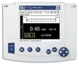
Figure 12. Display screen for IQ SensorNet UV-Vis spectrophotometer sensor
